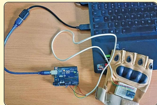
This Arduino-based gaming glove works like a mouse and keyboard in the air and allows you to control a graphic user interface (GUI).
